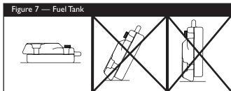
To place the fuel tank back on the unit, follow these same steps in reverse order. Make sure the four large plastic wing nuts are tightened securely.
